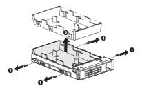
4 Align the new hard disk with the HDD carrier, then secure it with the four screws you removed in step 3-1.
